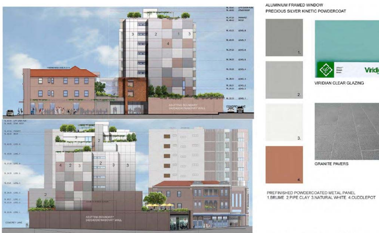
Figure 7 - Western Façade Materials and Finishes - Source ARC Architecture
